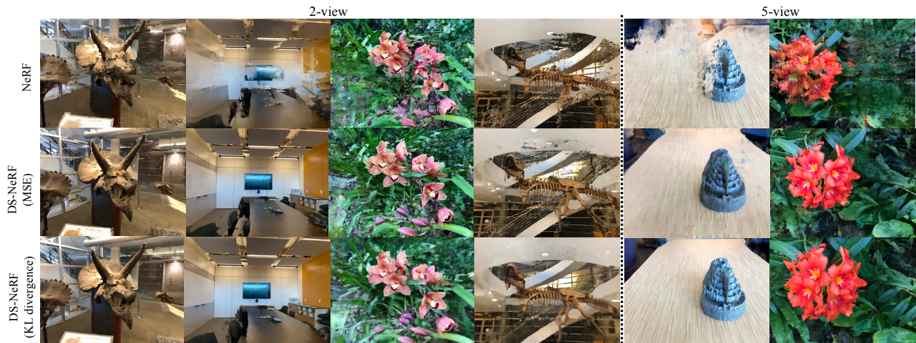
Figure 6. Depth Supervision Ablations. We render novel views for NeRF and DS-NeRF trained on 2 views and 5 views. NeRF fails to render novel views as evident by the many artifacts. Using MSE between rendered and sparse depth improves results slightly, but with KL Divergence, DS-NeRF is able to render images with the fewest artifacts.
